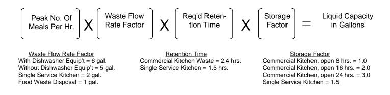
FOG interceptors must be installed on a separate building sewer line servicing kitchen flows and shall be connected only to those fixtures or drains which would allow fats, oils, and grease (FOG) to be discharged. This includes:
